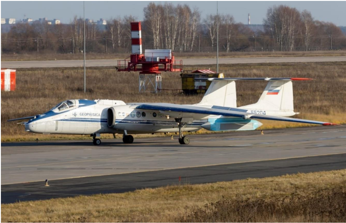
Figure 2: M-55 reconnaissance plane, equipped with the UKR-RL pod.
